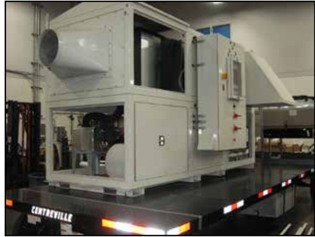
Figure 7.2.1.2-1. Portable Environmental Control System (PECS)
