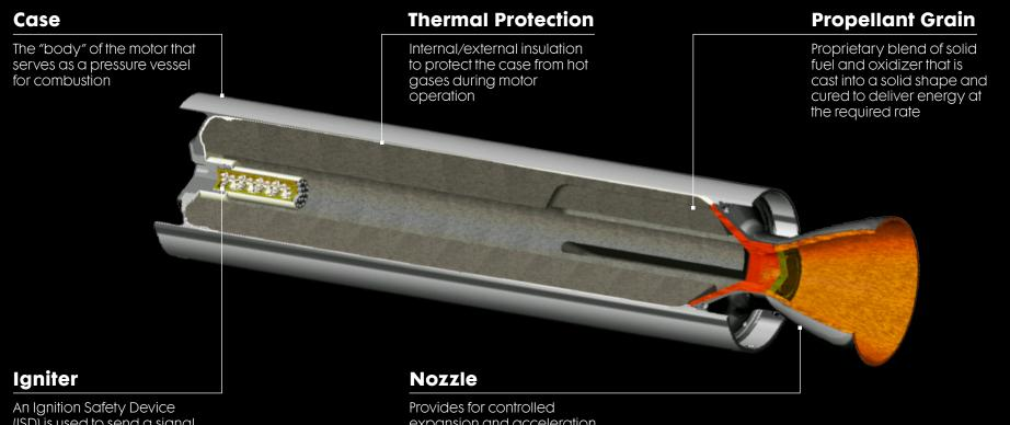
An Ignition Safety Device (ISD) is used to send a signal to the igniter, which ignites the solid propellant grain Provides for controlled expansion and acceleration of combustion gas, generating thrust for propulsion
