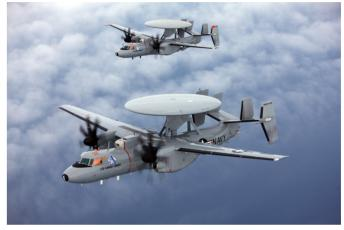
Northrop Grumman's AEW&C aircraft E-2D "Advanced Hawkeye" The U.S. Navy and the Japan Air Self Defense Force (JASDF) operate the aircraft. Its airborne radar covers hundreds of kilometers around. (Photo credit: U.S. Navy)
