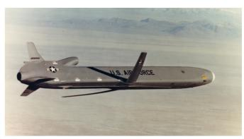
Boeing's AGM-86B ALCM cruise missile flying at a low altitude. Flight altitude is several tens to several hundred meters (Photo credit: U.S. Air Force)
