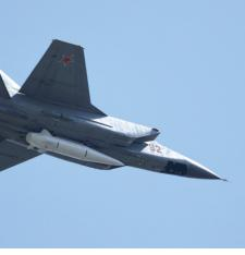
The hypothetical fighter jet and hypersonic weapon in this episode were based on the MiG-31 fighter and Kh-47M2 "Kinzhal" an air-launched hypersonic missile (carried under the fuselage). The missile is estimated to have a scramjet engine and flies more than hundreds of kilometers at hypersonic speed toward its target. (Photo credit: Toshiharu Suzusaki)
