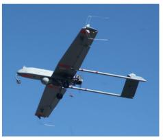
U.S. Marine Corps' RQ-7 Shadow UAV. Though having retired by the Marines in 2018, the tactical UAV's concept was to approach the enemy close to conduct electronic attacks while reducing human risk.
