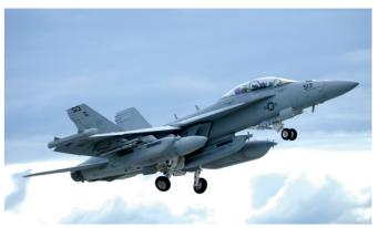
U.S. Navy's EA-18G Growler. The aircraft conducts various electronic attacks with the EW pods attached beneath the fuselage and at the wingtips. (Photo Credit: U.S. Navy)
