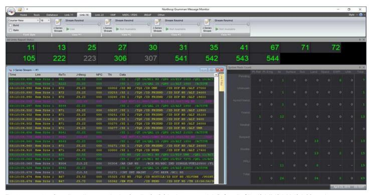
The Message Monitor allows the operator to view the individual message details for all of the Link 11, Link 16, Link 22, and JREAP messages that are being transmitted or received over the network. These messages can further be highlighted or filtered to show only the information needed, based on the users settings. All messages are shown in a common Data Extraction and Reduction Guide (DERG) format.
