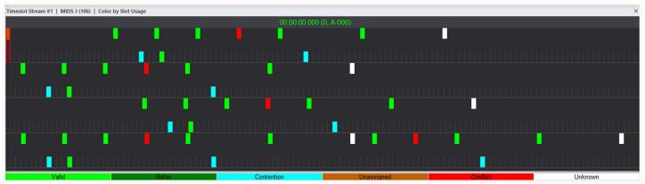
Multiple displays present a seamless tactical picture and summarize multi-TDL network performance. The operator can customize the display to include the most useful data — including signal quality and connectivity information — enabling an at-a-glance view of how networks are performing and which units are experiencing problems.
