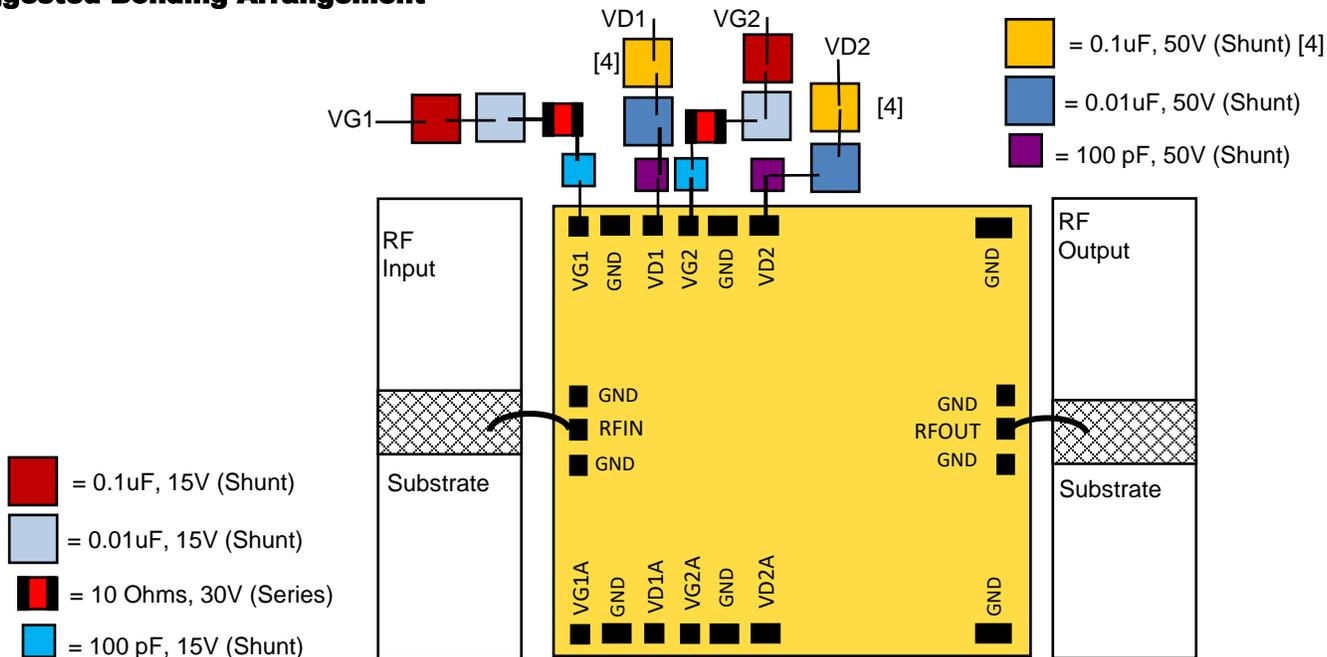
**Note:** APN226 can be biased from either the top or bottom and bias pads VG1A, VD1A, VG2A and VGD2A can be used as an alternative to the configuration shown.
