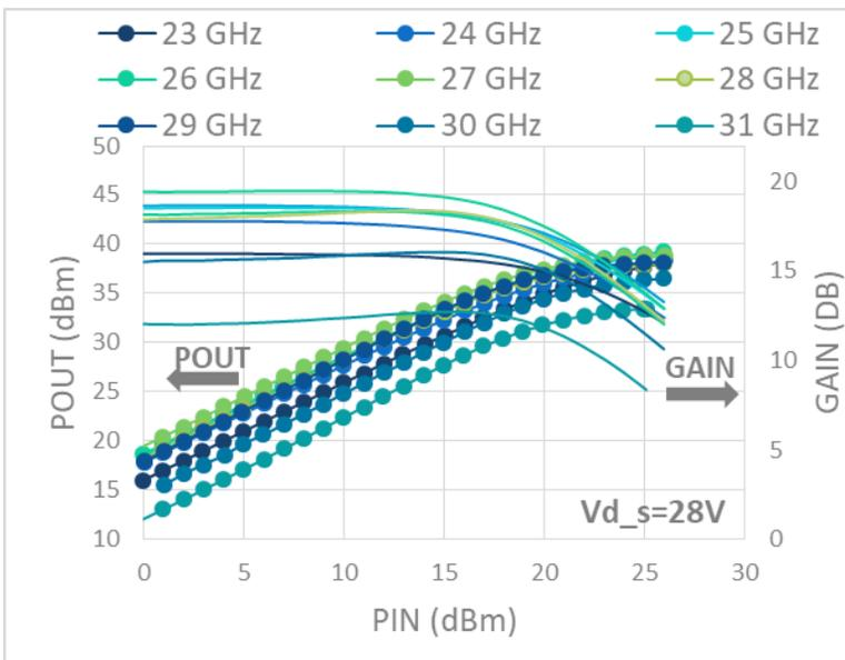
PAE, GAIN, POUT vs. FREQUENCY
