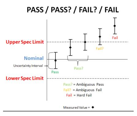
The graphic below illustrates how the TAR method of SOOT FAIL evaluation would compare to the uncertainty presentation of PASS / FAIL / FAIL? Results when the **FAIL\*=SPEC x** is modified to simulate 4:1 and 10:1 failures.
