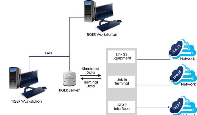
The above configuration can be used to inject simulated data, either ad hoc or via pre-scripted scenarios, from any TIGER workstation to any of the connected test networks. TIGER supports most TDLs, including Link 16/11/22, DIS, JREAP, and SIMPLE. All messages on the test networks, as well as the test Tactical Situation Display, are viewable on any TIGER workstation.
