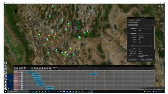
The Tactical Situation Display shows filterable track symbology. During test the user can switch between this window and the Message Monitor. The Message Monitor displays tactical messages, as well as scenario and operator-initiated events, in an organized, user-readable format.
