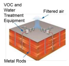
them to the surface where treatment equipment removes the VOCs. The filtered air is then released as noted in the light blue arrow on the illustration.
