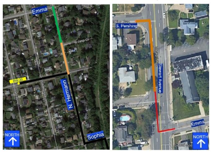
**ORANGE LINE IS CURRENT WORK ZONE; Black line is completed piping.**
